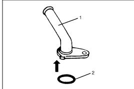
26) Install suction connector (2) to pump body as shown in figure. Tighten suction connector bolt (3) to specified torque.
